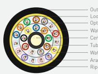
Outer Jacket Loose Tube Optical Fiber Water Blocking Yarn Central Strength Member Tube Filling Compound Water Blocking Tape Aramid Yarn Ripcord
