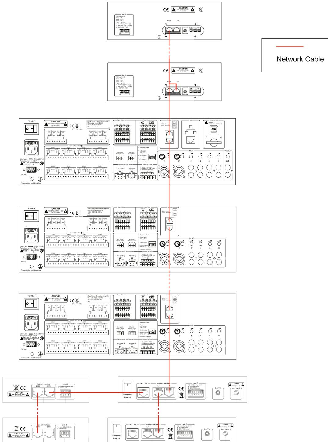
Instruction: The host NVS-50010508EV can connect up to 19 extended host NVS-50020508EV, and can 32 fireman MIC NVS-5004FM04EV and remote paging MIC NVS-5003PM16EV; among them, NVS-5007EX16EV is the extended remote paging device of NVS-5003PM16EV, and one NVS-5003PM16EV can connect to up to 9 NVS-5007EX16EV.
