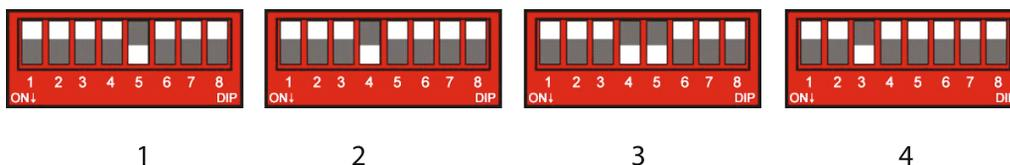
"6" and "8" is N/A, "7" is LED test, keep pulling up normally, pull down to enter LED test mode;
