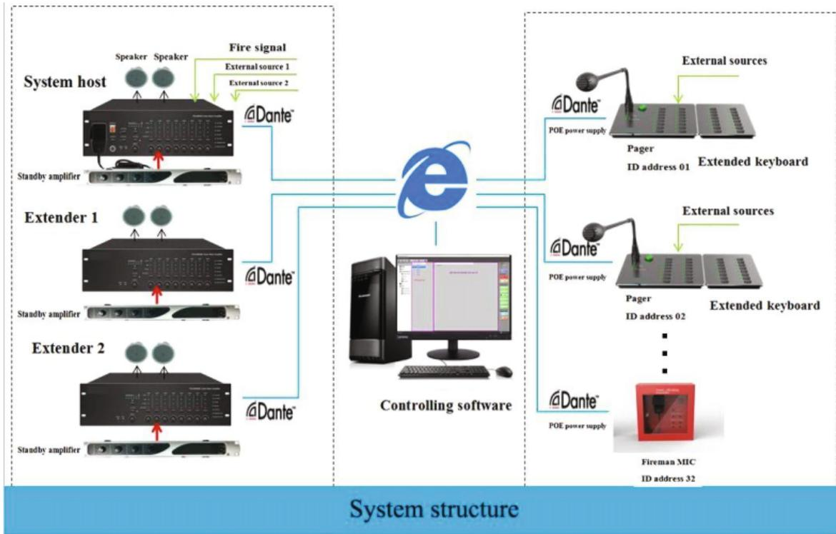
Instruction: Evacuation system is composed of system host NVS-50010508EV, extended host NVS-50020508EV, PC operation terminal, remote paging MIC NVS-5003PM16EV / NVS-5007EX16EV, MIC NVS-5004FM04EV. Data control and audio transmission are over Dante network. PoE powers remote paging MIC and Fireman MIC, which is compatible with the PoE power supply of the system host and of the PoE switch.
