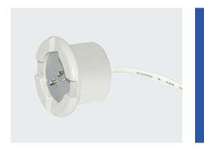
The water logging sensor can provide an output signal. When the water logging is high enough to reach at the sensor probes (about 1mm above the test surface), it sends an alarm signal.
