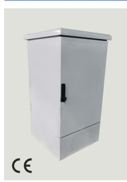
The Easycab range of floor Floor Standing cabinet IP 65 with 600W air condition is designed for external telecommunication purpose. The smart design and professional engineering provide easy installation and maintenance. It is comply with GB/T 19183 and IEC 61969 standards.
